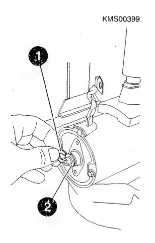
Checking and adjusting armature axial clearance
